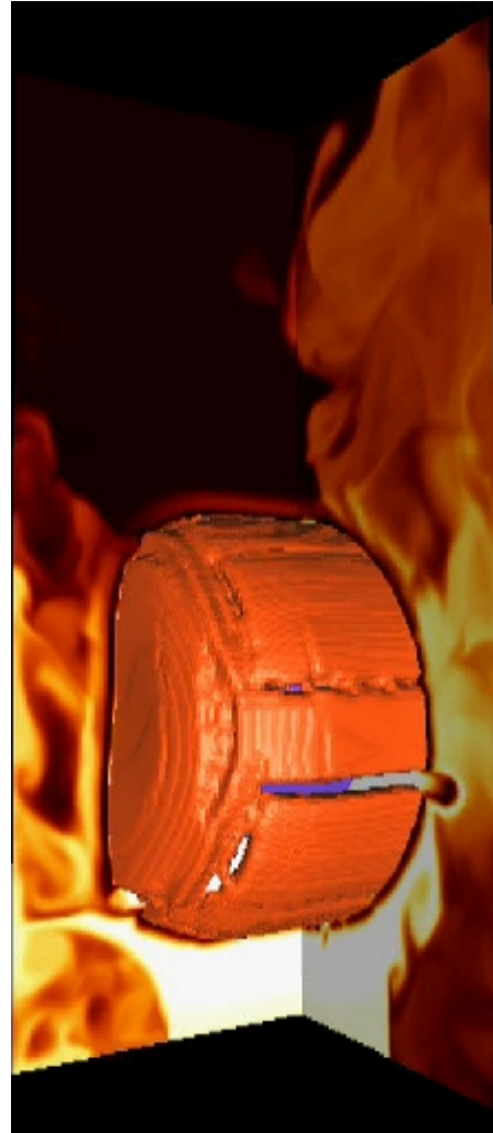
Figure 3: An example of contemporary visualization and simulation capabilities. Shown is a simulation of the explosion of a steel tank filled with explosive subjected to a jet of heated air. New methods are needed to capture multiscale effects and quantify uncertainties.
